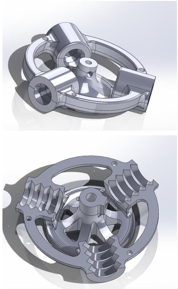
**Figure 13: CAD drawing of the tube connecting module**
